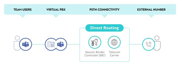
ZIRO's geographically and cloud meshed redundant architecture eliminat any single point of failure and provides greater than 99.99% availability. Private and secure voice transmission are encrypted using Transport Layer Security (TLS)/Secure Real-time Transport Protocol (SRTP).
